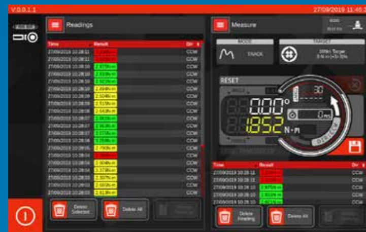
Readings pane (left) transducer measurement (right)
