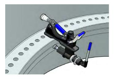
The tool has been designed to cope with the larger loads and dimensions associated with these flange joints while remaining relatively lightweight and user-freindly.
