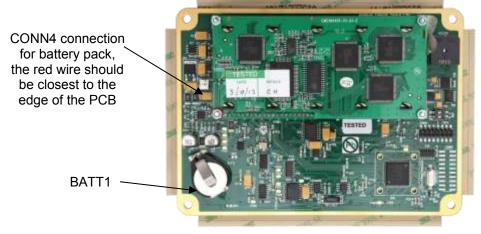
FIGURE 2 - PCB (Inside TTT)
