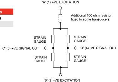
NOTE: The differential voltage output for STATIC and ROTARY transducers goes positive for clockwise torques, and negative for anti-clockwise torques.
