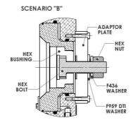
Figure 16, Calibrator Cross-section
