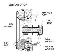
Figure 18, Calibrator Cross-section
