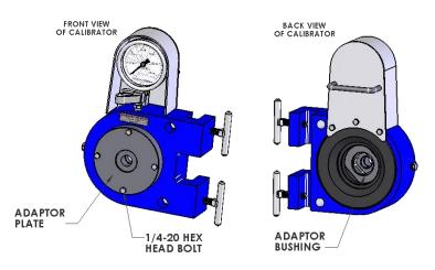
Figure 6, Installation of Adaptor Plate and Bushing
