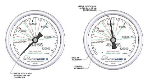
Figure 8, Example of How to Read Gage Dial
