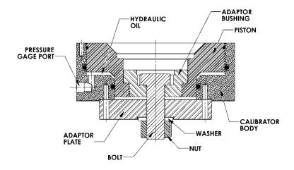
Figure 1, Typical Calibrator Cross-Section
