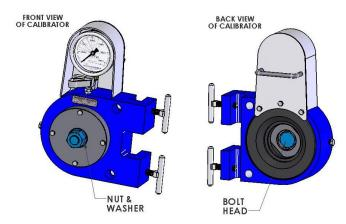
Figure 7, Installation of Fastener Assembly to be Tested
