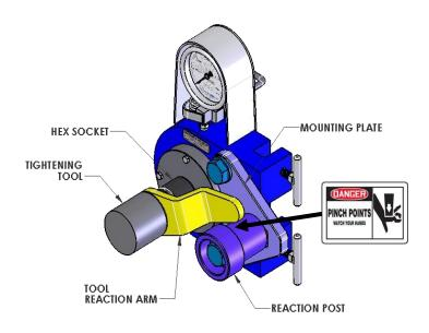
Figure 3, Typical Setup of Torque Reaction Kit
