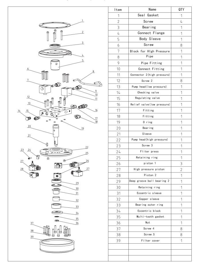
Part List with drawing for Valve Block
