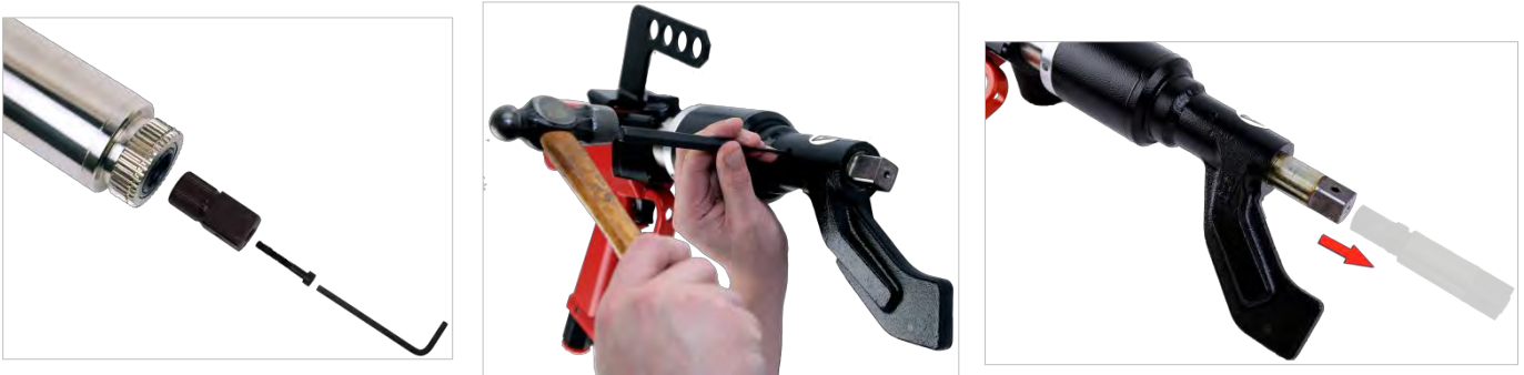
FIGURE 8 – Square Drive Replacement
