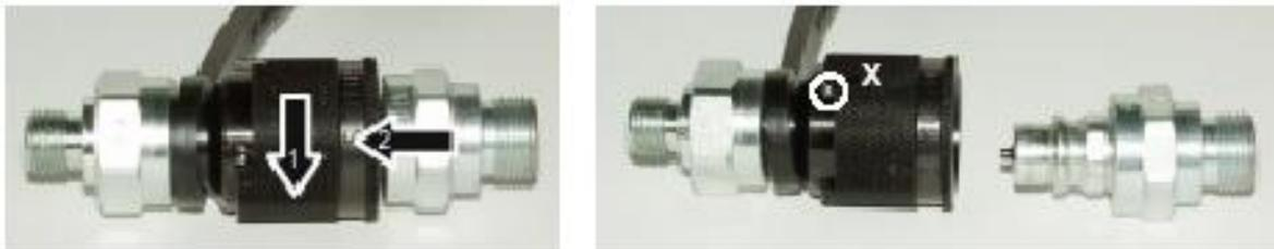
In position X, retract sleeve – plug and socket are uncoupled - the device is coupled in reverse order. The devices can only be coupled if the hose lines are **depressurized**.
